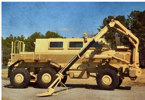
The Buffalo is a wheeled Mine Resistant Ambush Protected (MRAP) armored vehicle used to safely dispose of mines.
