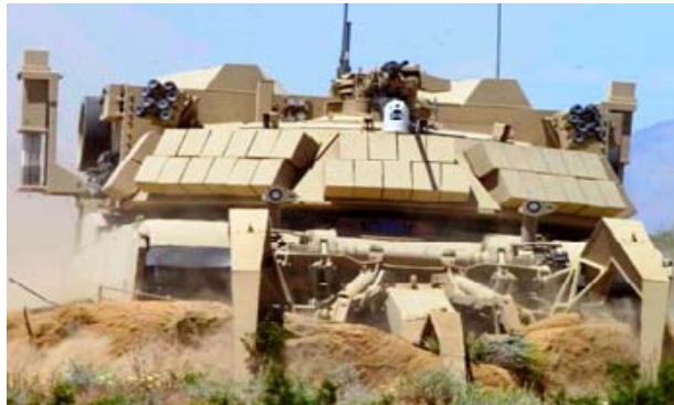
Assault Breacher Vehicle was designed to clear pathways for troops and other vehicles.
