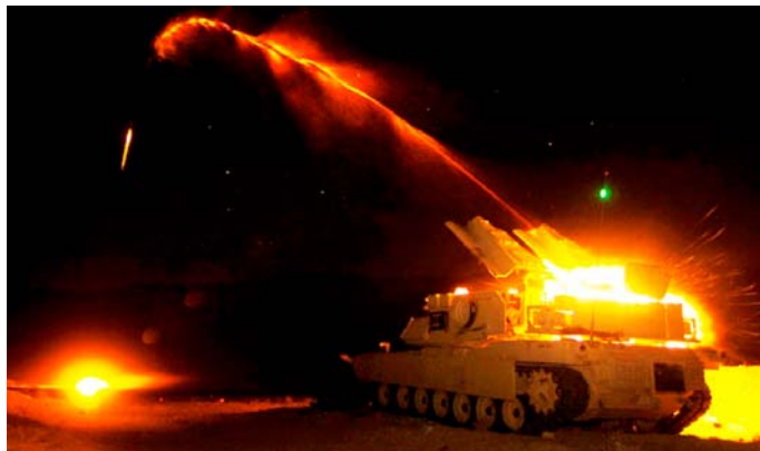
Assault Breacher Vehicle test firing an explosive line charge.
