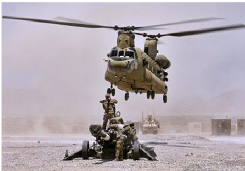
Soldiers hooked-up a M777A2 howitzer to a CH-47 Chinook helicopter for airlift.
